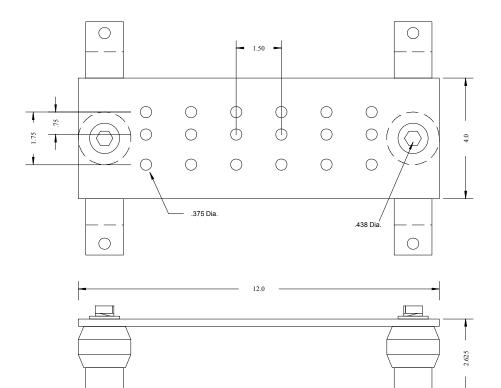
Standard busbar assemblies are insulated and specifically designed for commercial applications. The silver washed 110 alloy copper ground bars are 1/4" thick and stand off 2.625" from the wall or backboard.
